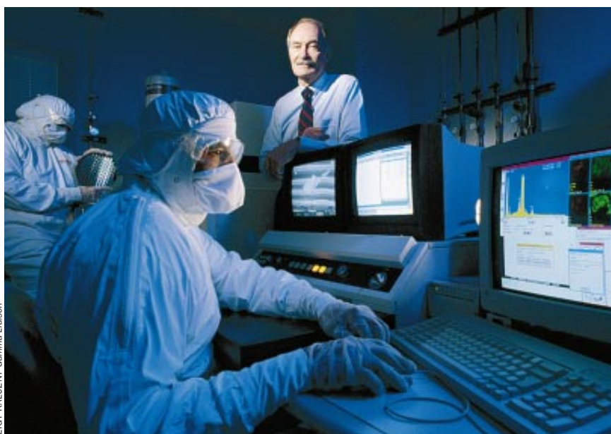
SEMATECH PRESIDENT William J. Spencer poses in the consortium's chip-inspection laboratory. Workers are in clean-room suits to prevent dust and other contaminants from reaching silicon wafers and equipment. An electron microscope image of an integrated circuit is visible on the monitor screen at the right.
